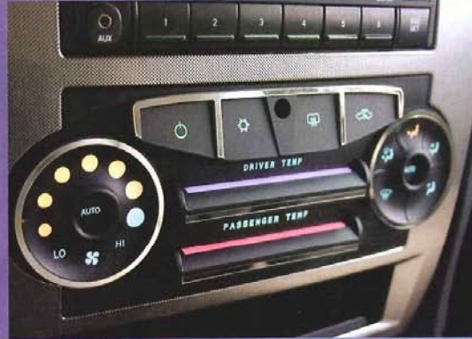
TRW's capacitive switches provide flat surfaces that feature lighting and haptics.
