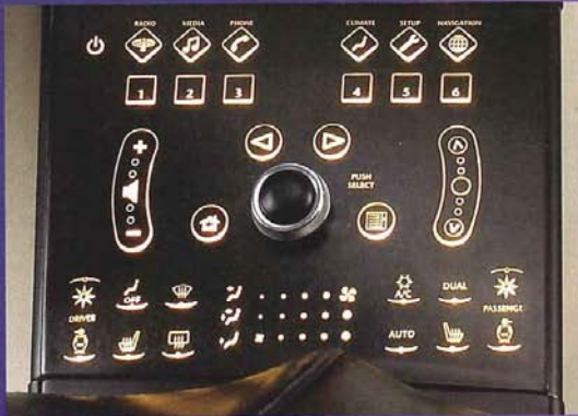
Visteon controls light up when a hand gets near the control panel.
