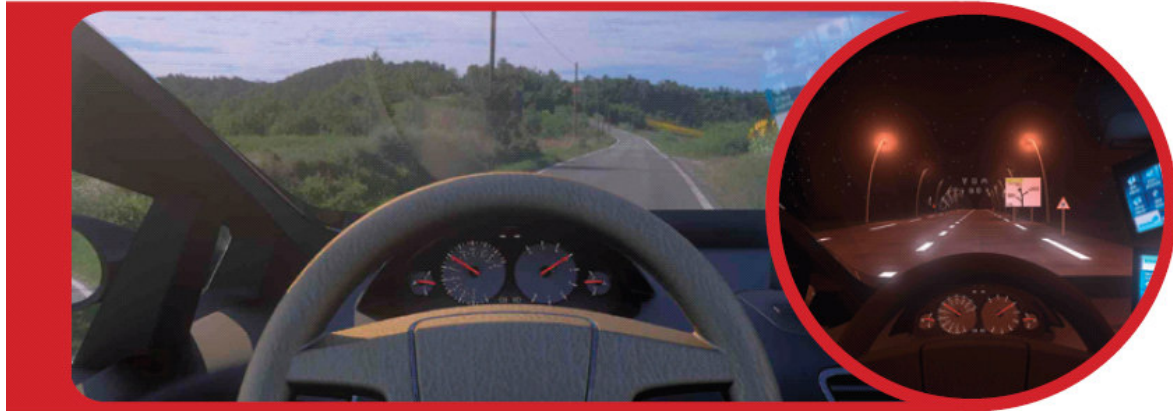
LEFT: Simulated in OPTIS software : GPS Screen as it would be visible with oncoming sun. RIGHT: Simulated in OPTIS software : unwanted reflections of dashboard screens in windshield.
